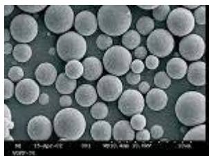
Superparamagnetic silica particles (ferrofluid encapsulated in tetra methoxy silane) (left) and hydrophilic acrylate particles from HEMA/N,N-methylene bis-acrylamide (right)
